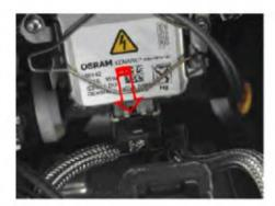
The factory harness routing may cause too much tension on the HID Bi-Xenon headlamp connector. When adaptive action (movement) is enabled, the HID Bi-Xenon headlamp wiring harness may disconnect from the HID Bi-Xenon bulb connector.
