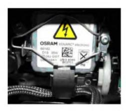
Install the affected HID headlamp assembly. See Repair Manual Group 94 - Lights, Switches - Exterior.
